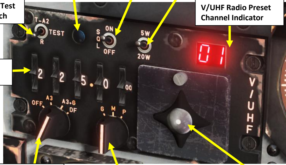
V/TVU-740 V/UHF Radio Function Selector • OFF • A3: Transmit-Receive • A3+G: Transmit-Receive + Guard • DF: Directional Finding
